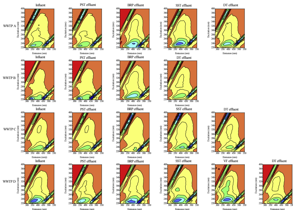
Fig. 6. Fluorescence spectra for DOM in influents and different treatment unit effluents of the four WWTPs.
